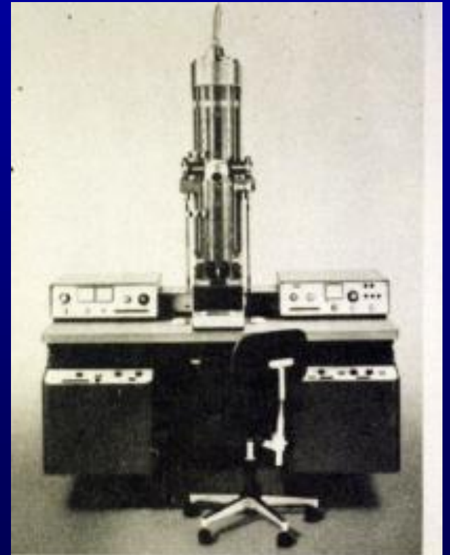
Figure 1-5. Photograph of the Zeiss model EM 10 electron microscope. (Courtesy of Carl Zeiss Co.)
