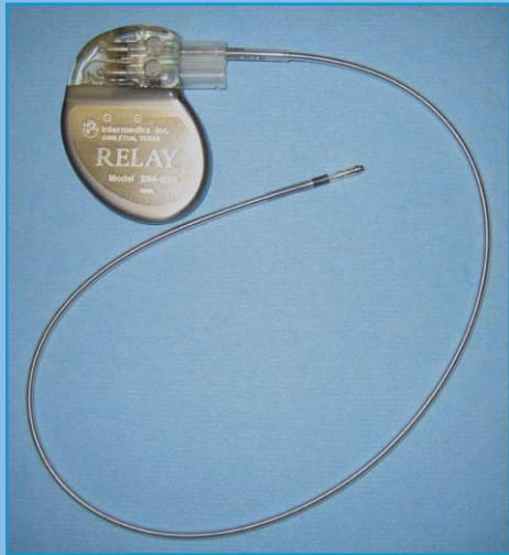
A pacemaker is made up of two components: a battery and a lead.
