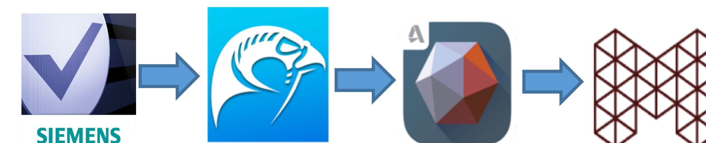
Fig. 8) Multiple softwares were used during the whole process to transform the medical DICOM images into the 3D printed models. The average time of post-processing took about 1 hour, depending on the complexity of the desired target.
